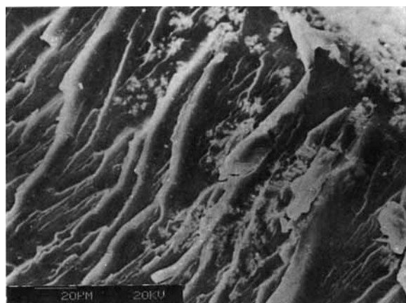
Figure 7 Morphological structure of transition layer of ECCF from SEM. Concentration of PAN to DMF in PCBS: 17% (wt); ratio (mole/mole) of nitrile group to copper(II) ion: 2 : 1; drying time of SSF: 16 h; current: 0.8 A; reaction time: 2 h.
